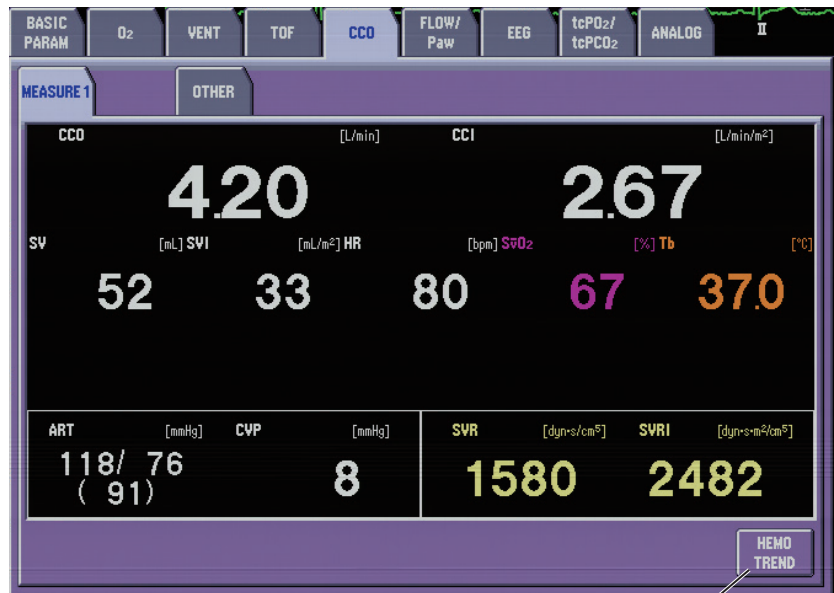
Displays the hemodynamics table on the HEMO TREND page of the TREND window
